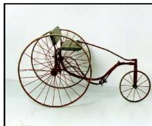
#171R Child's treadle tricycle, 2 x 26" solid rubber tyred rear wheels, 12" front wheel, maybe as early as 1888. $2000 neg.
