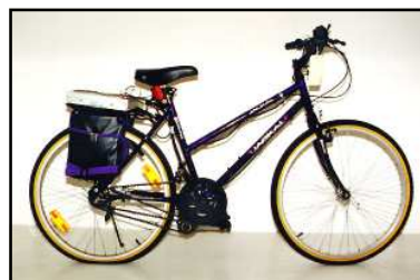
#537 Solar Elektra Mobil fitted on standard Recco 26" bike, with added solar panels and batteries in rear panniers. Assembled in Sydney 1994. $300
