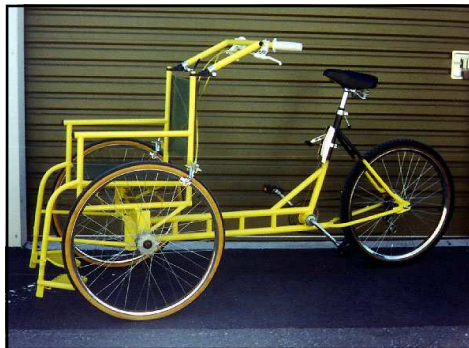
#446 PWD tricycle 26" & 24" wheels. Chair in front, pedaller behind. Built by Toowoomba Bicycles 1991. $300
